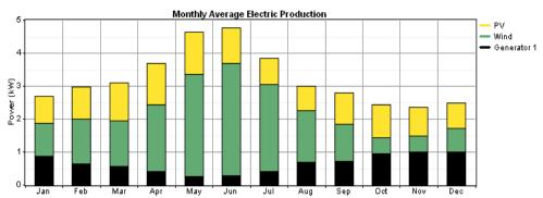
Figure 16. Nema (2010) Average monthly electricity production of a hybrid energy supply system
