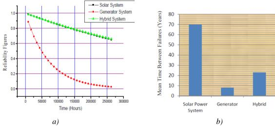
Figure 8. Faruk (2012) a) Reliability of hybrid power system and b) Mean time before failure
