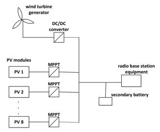
Figure 10. Configuration of autonomous power supply system
