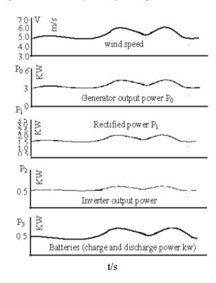
Figure 5. (Yiming, 2009) Simulation results obtained using the MatlabSimulink tool
