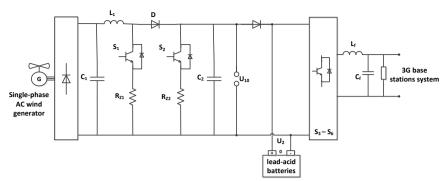
Figure 4. Control system of wind powered BS site
