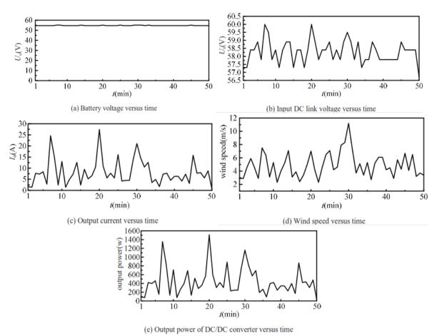
Figure 3. (Shuang, 2011) a) Battery voltage, b) Iput DC link voltage, c) Output current, d) Wind speed, and e) Output power of a DC/DC converter during intervals of fifty minutes
