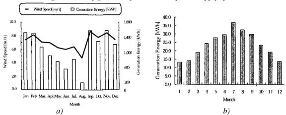
Figure 11. Hashimoto (2004) a) Monthly wind speed and wind turbine energy generation, and b)
