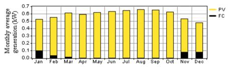
Figure 14. (Bazmalinovic, 2013) Averaged monthly electricity production of power supply system based on PV modules and fuel-cells
